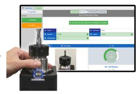
ToolConnect validates the tool length being loaded into the machine. In this case, where the tool was longer than it should have been due to a measurement error, ToolConnect would have prevented the tool from being registered in the machine and forced the operator to intervene.
