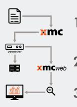
Raw data enters the XMC<sup>®</sup> platform through the machine tool, plus any barcoders, sensors, or other sources you may utilize. Usually, no additional hardware is required.
