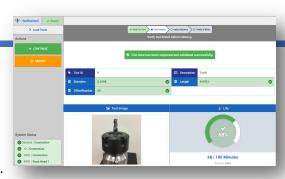
The operators no longer manually enter the tool data, it happens automatically. ToolConnect reads and updates all geometry and wear offsets to the control. As an added failsafe, if an operator tries to load an incorrect tool, or a tool in the wrong pot, ToolConnect will alert the operator.
